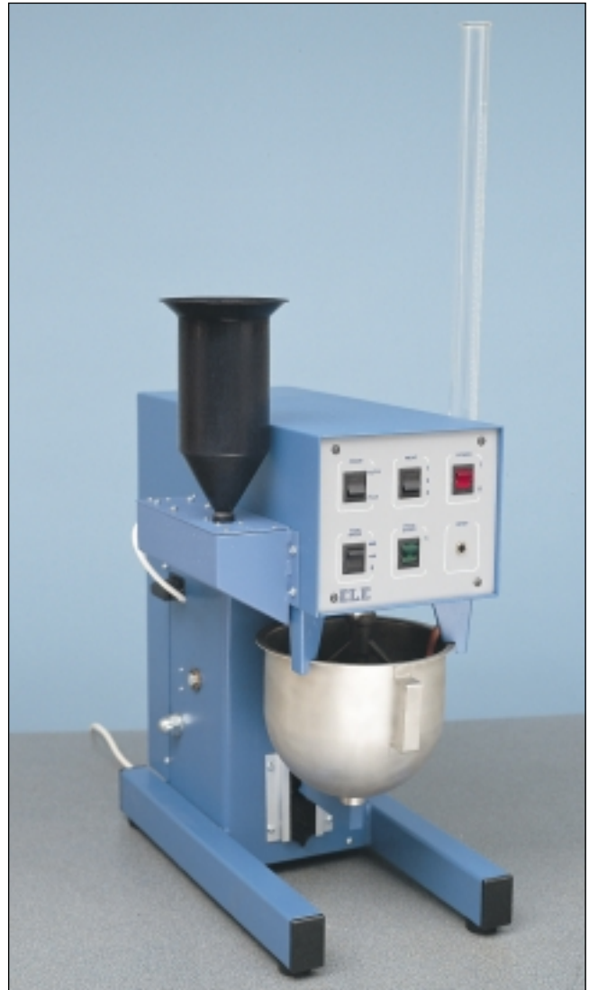
EL39-0031/01 Automatic/Manual 5 litre (nominal) Mortar Mixer with Accessories
